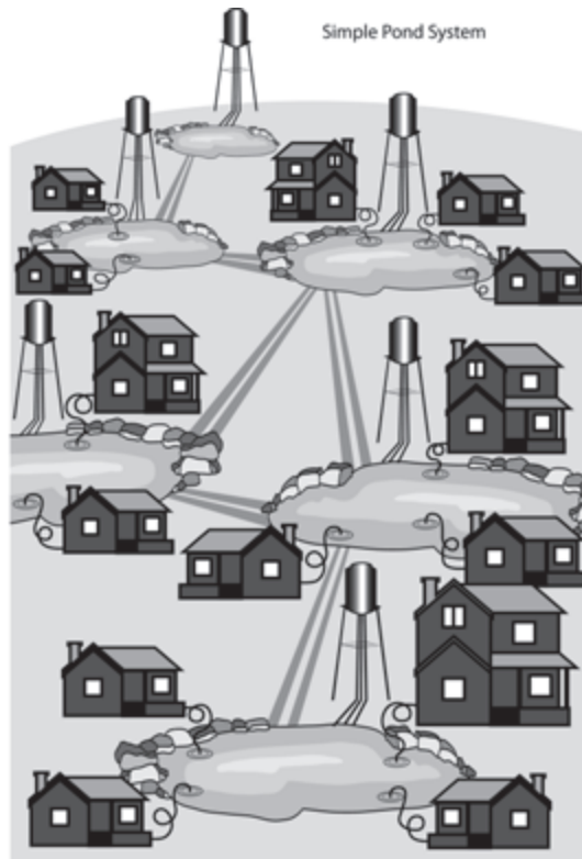
Figure 3-1. The Pond System Analogue to the Power Grid.
