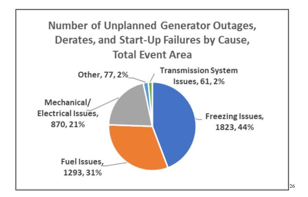
Their report identified 44% of unplanned outages, derates, and startup failures as being caused by freezing. They further contended that an "analysis of the 21% of outages, derates or failures to start caused by 'Mechanical/Electrical Issues' indicated that they are also related to the cold temperatures."<sup>27</sup> The report also suggested that almost a third of outages were due to fuel issues.<sup>28</sup>
