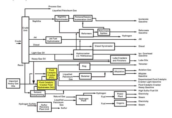
Richmond produces gasoline components in two different production sequences. The August fire took place at the other production process, crude unit #4, depicted as the long rectangle at the upper left part of the plant flow chart. The May report indicated a two week interruption in the second production sequence.
