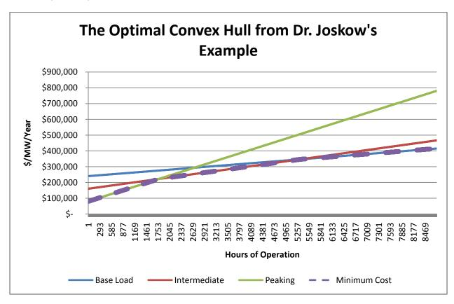
The least expensive result for each hour is represented by the dashed line which shows the best choice of resource for each level of expected operations. Not surprisingly, in this example, peakers are optimal for operations over a small number of hours (1 through 1,777), intermediate resources dominate from 1,778 through 5,343 hours a year, and base load units are best for longer durations (5,334 hours through 8,760 hours a year).
