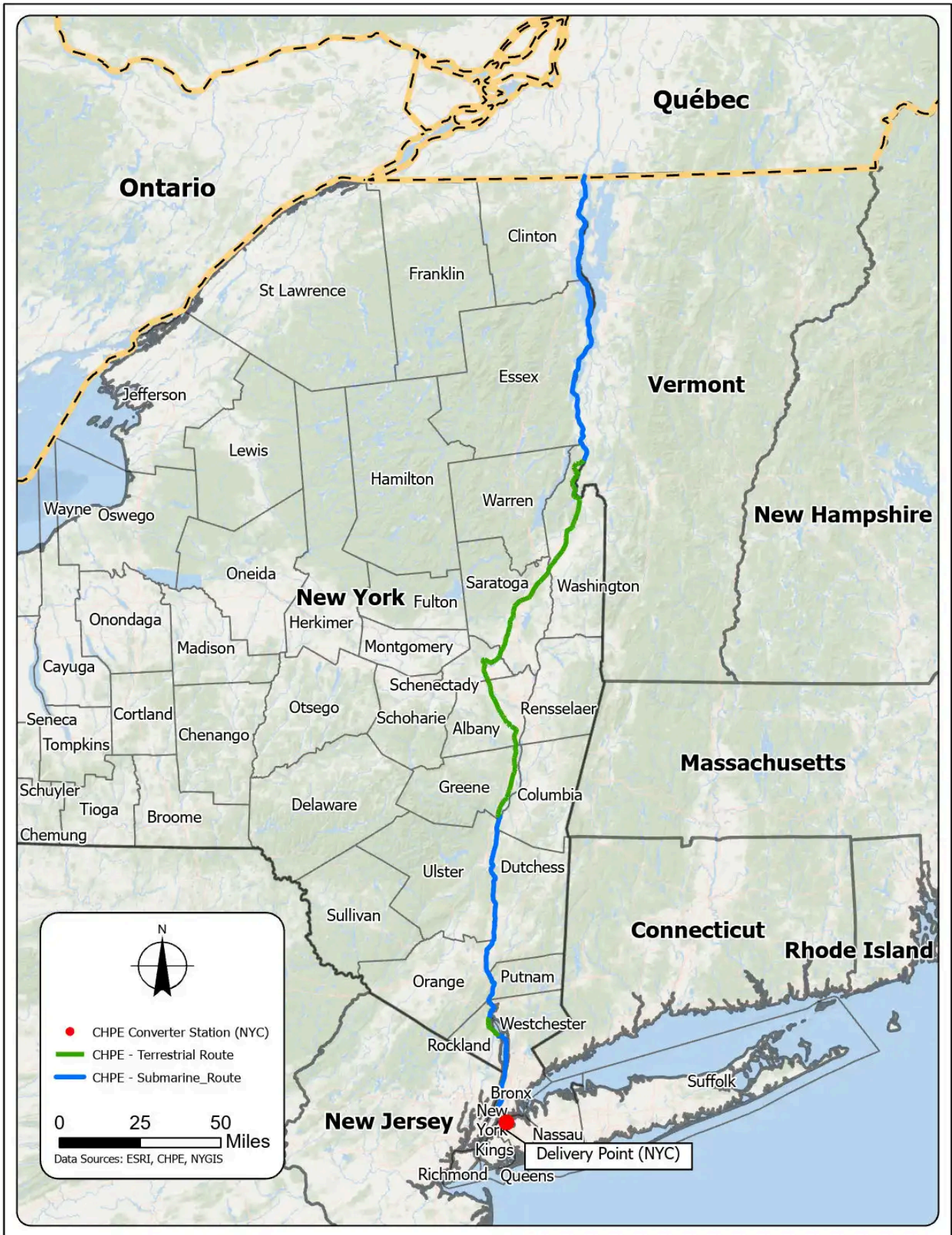
The new Champlain Hudson Power Express (CHPE) line runs from Quebec down to New York City, including stretches beneath Lake Champlain and the Hudson River. Courtesy TDI CHPEXpress
