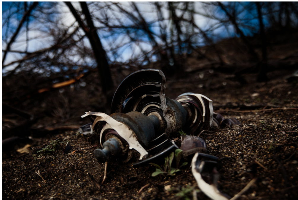
A broken insulator underneath a PG&E transmission line outside the town of Pulga, Calif. Max Whittaker for The New York Times
